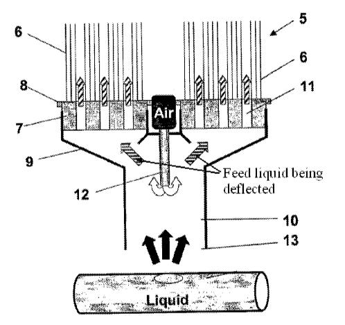
Heine in view of Shimizu fails to disclose or suggest a gas inlet constructed and arranged to introduce gas into a mixing chamber in a downward direction from above the open base end, said gas fed from above and through said clover-type manifold
